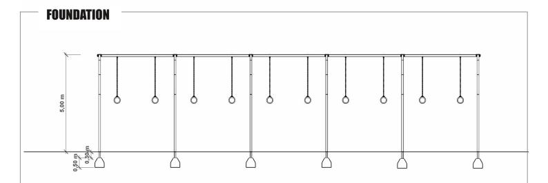
Each vertical column and steel wall anchor poured with semi-dry concrete C20/25 for 80 cm below ground level. Volume of one footing min. 0,125 m3 (50x50x50 cm). Fundations are placed 30 cm below ground level, what prevent accidential or purposeful discovery.
